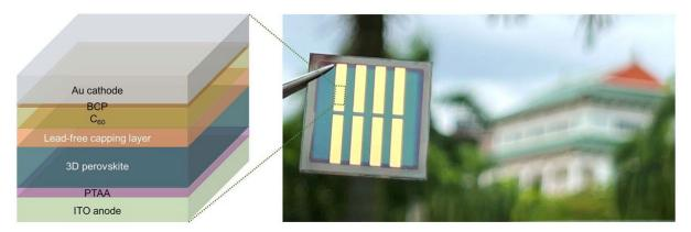
"One of the biggest drawbacks of using perovskite solar cells is their impact on the environment. By allowing zinc and other non-toxic metals to be used in the cover layer, our innovation potentially solves a major barrier preventing the use widespread use of perovskite solar cells," said Dr. Ye Senyun, a researcher at NTU's School of Physical and Mathematical Sciences, one of the study's lead investigators.
